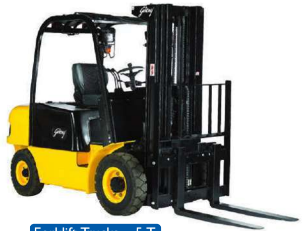
Forklift Trucks - 5 T.
