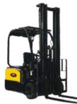
3 wheel Forklift - GX Series 0.8 to 2 tonne
