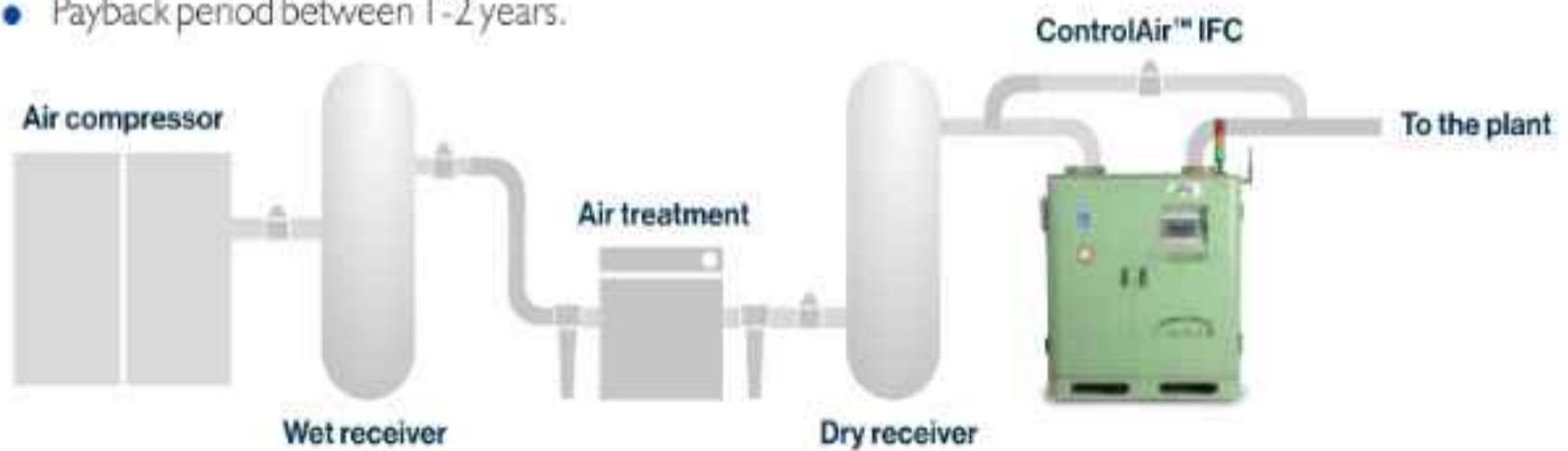
Typical Installation of IFC in a Compressed Air System
